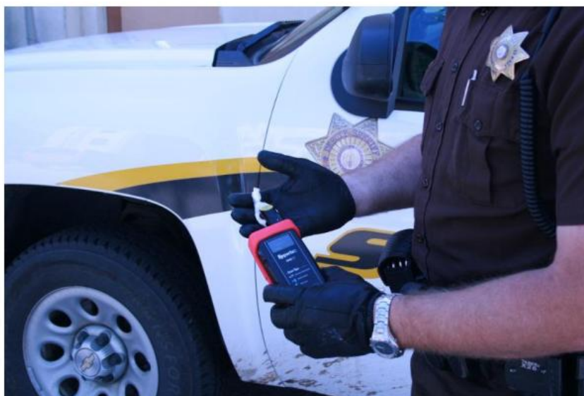
Intevac Photonics' Reporter™ hand-held Raman systems use wavelength stabilized lasers for rapid identification of unknown narcotics in the field.
